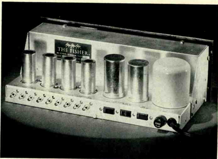
Rear view of the 80-C "Master Audio Control." Shielding is used extensively.
